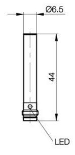
Inductive Sensors BES 516-3021-G-E5-C-S 49 D6.5 x 44 normally-closed Sn=2mm shielded
